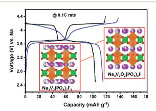
Fig. 12 Charge/discharge curves of  $Na_3V_2(PO_4)_2F_3$  in black and  $Na_3V_2O_2(PO_4)_2F$  in blue for SIBs. Both structures show the connectivity of  $VO_6$  (orange) octahedra and  $PO_4$  (green) tetrahedra along the [010] direction. The pink, red, and silver balls represent sodium, oxygen, and fluorine, respectively.
