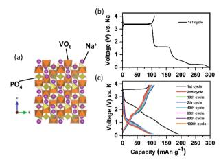
Fig. 10 (a) Structural diagram of  $Na_3V_2(PO_4)_3$ ; charge/discharge curves of the carbon coated  $Na_3V_2(PO_4)_3$  composite in the (b) SIB and (c) PIB.
