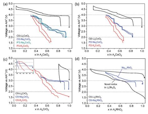
Fig. 5 Typical charge/discharge profiles of (a) O3 and P(')3 type  $A_xCoO_2$ , (b) O2 and P(')2 type  $A_xCoO_2$ , (c) O3 type  $A_xCrO_2$  with an inset for those cycled in higher upper cut-off voltage, and (d) O3 type  $A_xRhO_2$  in non-aqueous Li, Na, and K cells. Filled circle represents a starting point of charge.
