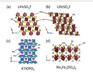
Fig. 11 Typical compounds representing (a) tavorite, (b) triplite, (c)  $KTiOPO_4$ , and (d) alluaudite types.
