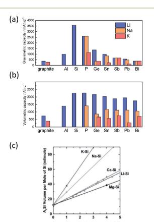
Fig. 21 Theoretical (a) gravimetric and (b) volumetric capacities of selected alloy materials for LIBs, SIBs, and PIBs. The volumetric capacities were calculated at the fully charged state. (a) and (b) are adopted with permission from ref. 4. Copyright 2020 American Chemical Society. (c) Volume of A<sub>x</sub>Si per mole of Si plotted as a function of the charge stored. Reproduced with permission from ref. 303. Copyright IOP Publishing
