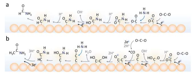
Fig. 7 Plausible surface reaction pathways in the electrosynthetic process of formamide (a) and acetamide (b) generation. Formamide generation depends on  $NH_3$  coupling with the first reaction intermediate while acetamide generation requires highly reduced  $C_2$  intermediates to be present on the catalyst surface. For simplicity, the donation of a proton to surface intermediates  $via\ H_2O \to OH^-$  is depicted as  $\to H^+$ .
