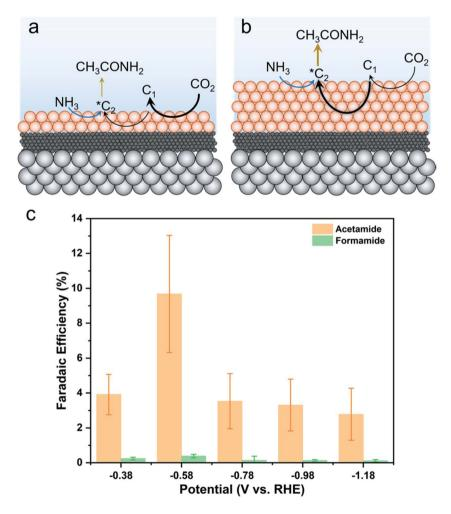
Fig. 6 A thicker catalyst loading was found to promote acetamide formation. Thin layers tend to form  $C_1$  products at a greater rate (a) while increasing the layer thickness leads to further reduction and accumulation of  $C_2$  intermediates that can be used for C–N bond formation (b). As such, an optimized Cu loading of 10 mg cm<sup>-2</sup> resulted in up to 10% acetamide selectivity (c).
