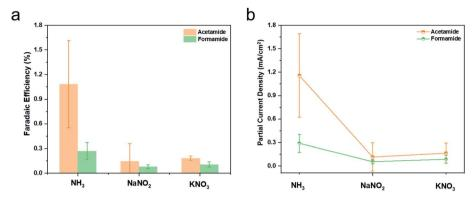
Fig. 5 In the equivalent reaction setup as in Fig. 3 with Cu catalysts and  $NO_2^-$  (0.5 M) or  $NO_3^-$  (1 M) in place of  $NH_3$  at -0.98 V vs. RHE, formamide and acetamide were generated. The faradaic efficiencies (a) and partial current densities (b) for their generation were compared to those from using  $NH_3$ .
