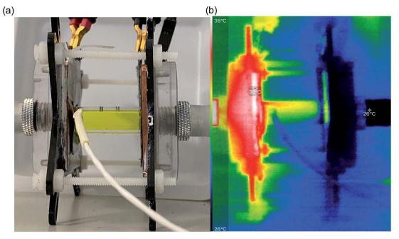
Fig. 4 Photos of (a) the actual thermogalvanic cell, sandwiched between the two heat exchangers (the white wire coming from the left is the heat flux sensor wiring); electrode separation = 29.3 mm,  $\Delta T_{app}$  = 20 K; and (b) IR image of the same cell, going from white = hottest to black = coldest
