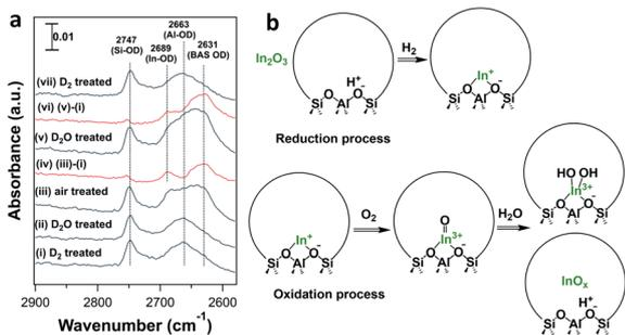
Fig. 8 (a) FTIR spectra of reduced In-CHA(11, 1.0) treated under different conditions at 550 °C: (i) D<sub>2</sub>; (ii) D<sub>2</sub>O; (iii) air; (iv) (i) subtracted from the spectrum (iii); (v) D<sub>2</sub>O; (vi) (i) subtracted from the spectrum (v); (vii) D<sub>2</sub>O. Background spectrum was collected in the spectral cell with the H<sub>2</sub> reduced sample pellet at 550 °C. (b) Proposed structures of exchanged In species in In-CHA upon reduction and subsequent oxidation.
