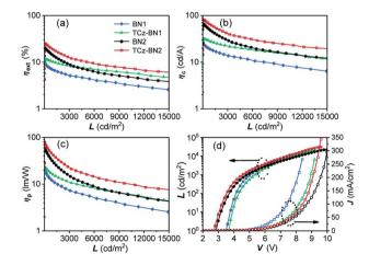
Fig. 7 EL characteristics of OLED devices based on BN1, TCz-BN1, BN2 and TCz-BN2. (a) The external quantum efficiency ( $\eta_{ext}$ ), (b) current efficiency ( $\eta_c$ ) and (c) power efficiency ( $\eta_p$ ) versus luminance (L) curves for the devices; (d) luminance (L)-voltage (V)-current density (J) characteristics for the devices.
