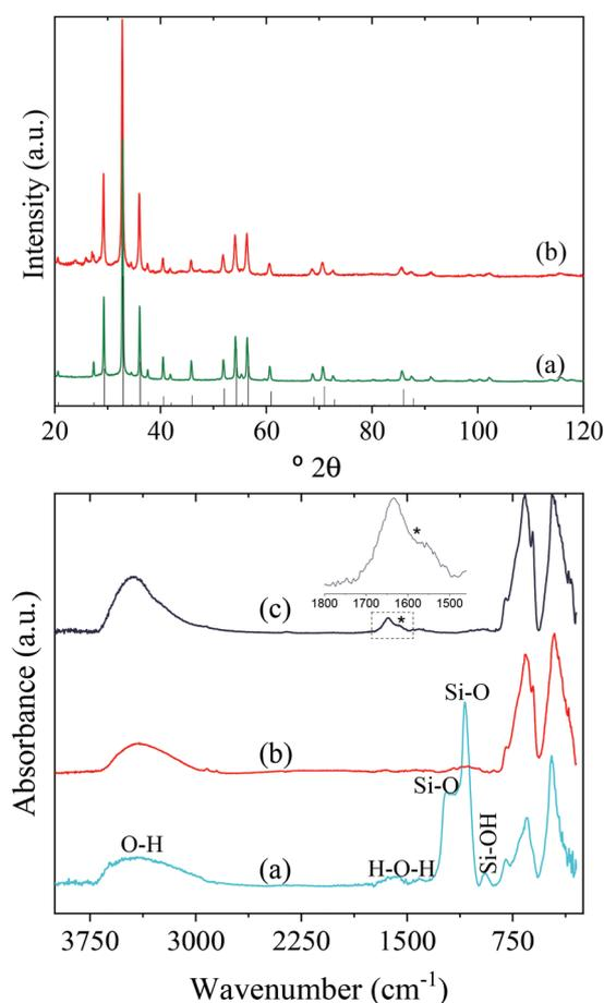
**Fig. 2** Top: XRD patterns of the AP-NPs (a) and C-NPs (b) together with the reflections corresponding to  $Y_3Al_2Ga_3O_{12}$  garnet (PDF 01-075-0556). Bottom: FTIR spectra of the AP-NPs@SiO<sub>2</sub> (a), C-NPs (b), and C-NPs@PAA (c).
