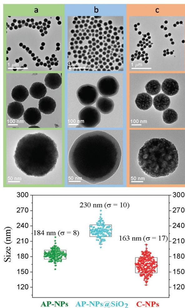
**Fig. 1** Top: TEM micrographs recorded at different magnifications of (a) as-prepared NPs (AP-NPs), (b) AP-NPs covered with a silica shell (AP-NPs@SiO<sub>2</sub>), and (c) AP-NPs@SiO<sub>2</sub> after calcination and HF washing (C-NPs). Bottom: Size distribution curves obtained from the TEM micrographs of the AP-NPs (green dots), AP-NPs@SiO<sub>2</sub> (blue dots), and C-NPs (red dots).  $\sigma$  stands for standard deviation.
