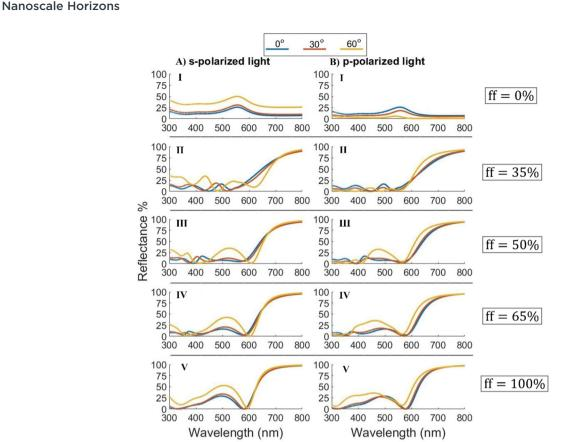
Fig. 6 Reflectance profile for a nanosheet HMM of different metal fractions with different angles of incidence. Color coding of curves correspond to indicated angles of incidence in the top box of the figure. Curves calculated for a hexagonal NP array above a Aq/TiO2 multilayer HMM stack, with all other parameters as in Fig. 4, for the Ag fill fraction as indicated in each panel.
