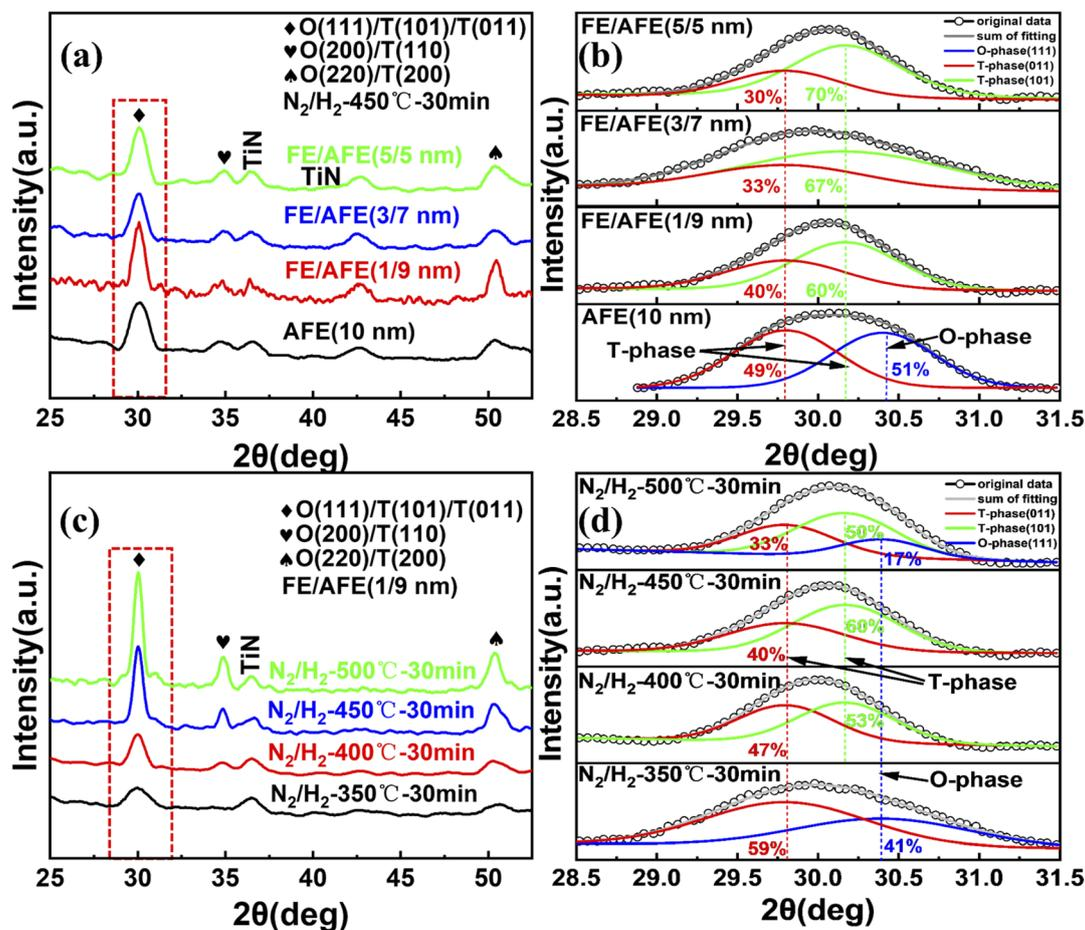
Fig. 4 (a) GIXRD patterns and (b) de-convolution of the diffraction peak of O (111)/T (101)/T (011) for the single AFE film and different FE/AFE stacks on the TiN film after annealing at  $450^\circ\text{C}$  for 30 min; (c) GIXRD patterns and (d) de-convolution of the peak of O (111)/T (101)/T (011) for the FE (1 nm)/AFE (9 nm) stack on the TiN film after annealing at different temperatures for 30 min.
