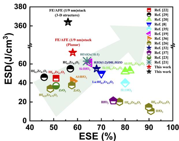
Fig. 9 Comparison of the achievable ESD and the ESE between our FE/AFE stack capacitors and other HfO<sub>2</sub>/ZrO<sub>2</sub>-based single AFE capacitors.
