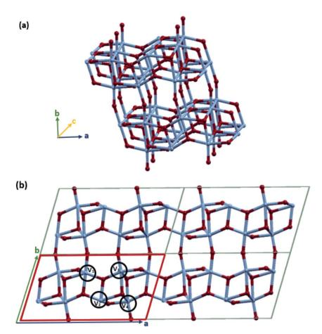
Fig. 1 Schematic representations of (a) the 3D frameworks of VO<sub>6</sub> octahedra in VO<sub>2</sub>(B) (b) 2D  $2 \times 2$  supercell of the VO<sub>2</sub>(B) polymorph, solid red line represents the unit cell of the structure. Color code in the model: V blue and O red.
