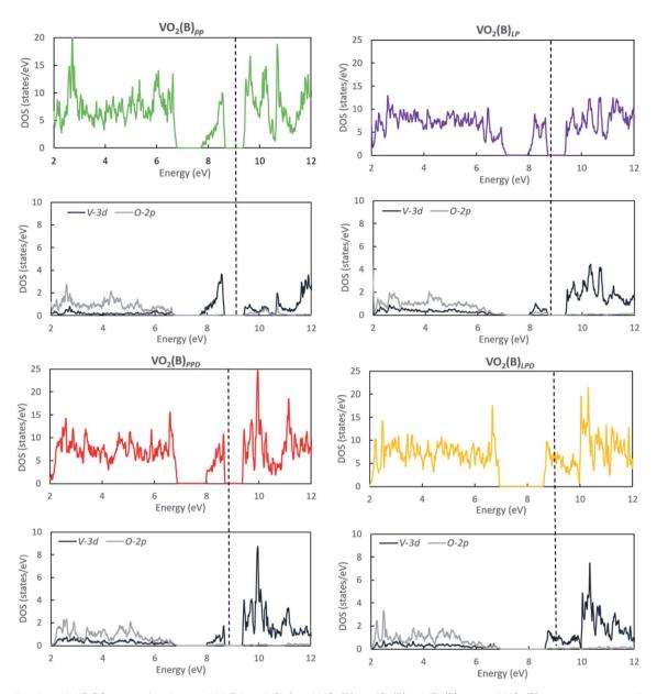
Fig. 3 Total and partial DOS curves for the total, V-3d, and O-2p of  $VO_2(B)_{PP}$ ,  $VO_2(B)_{LP}$ ,  $VO_2(B)_{PPD}$ , and  $VO_2(B)_{LPD}$  structures predicted by the GGA/PBE + U functional. Fermi energy aligned in the dash line.
