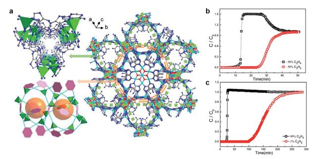
Fig. 6 (a) The channel and cavities in the 3D structure of NbU-1. (b) and (c) Breakthrough experiment for the mixture of  $C_2H_2$  and  $C_2H_4$  (50 : 50, 1 : 99, respectively). From the mixture of  $C_2H_2$  and  $C_2H_3$  and  $C_2H_4$  (50 : 50, 1 : 99, respectively).
