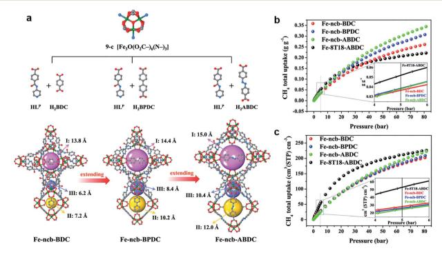
Fig. 5 (a) The constructions of Fe-ncb-MOFs. (b) The CH<sub>4</sub> gravimetric adsorption isotherms at 298 K. (c) Volumetric adsorption isotherms at 298 K.51 Reproduced from ref. 51 with permission, copyright The American Chemical Society, 2021.
