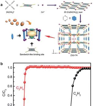
Fig. 8 (a) The construction process of ZJU-74a, 3D framework, and sandwich-like binding sites. (b) Experimental column breakthrough curves for a 1/99 C<sub>2</sub>H<sub>2</sub>/C<sub>2</sub>H<sub>4</sub> mixture at 298 K and 1 bar.<sup>68</sup> Reproduced from ref. 68 with permission, copyright John Wiley and Sons, 2020.
