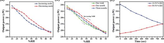
Fig. 7 Humidity measurement for investigating (a) repeatability, (b) aging effect with increasing % RH value from 10 to 90 and (c) response and recovery times of ZNR1
