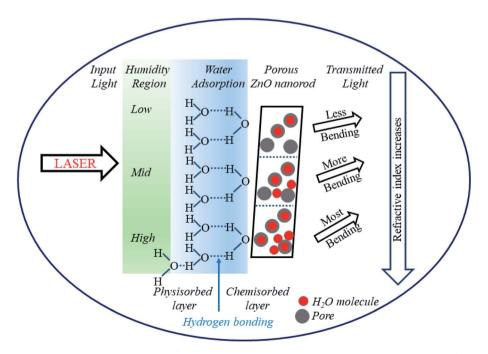
Fig. 6 Schematic of the sensing mechanism showing a decrease in output power with an increase in % RH for ZnO nanorods.
