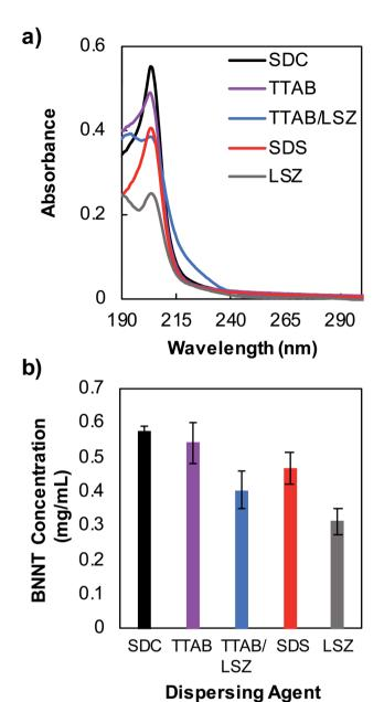
**Fig. 1** Dispersions of pristine BNNTs in water stabilized by various dispersing agents including SDC, TTAB, TTAB/LSZ, SDS, and LSZ. (a) Absorbance spectra of supernatant dispersions of BNNTs and the corresponding (b) concentration of dispersed BNNT complexes. All samples were diluted by a factor of  $200\times$  in DI water for UV-vis absorbance measurements. The error bars were obtained from the standard deviation of a minimum of three repeats of different dispersion samples.
