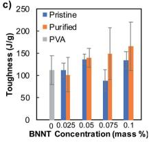
Fig. 2 Mechanical properties including (a) tensile strength, (b) Young's modulus, and (c) toughness of neat PVA (i.e., PVA), pristine BNNTs/PVA (i.e., pristine), and purified BNNTs/PVA (i.e., purified) fibers produced from dispersions containing 5 mass% PVA and varying BNNT concentrations in an EtOH coagulation bath.
