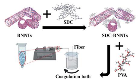
Scheme 1 BNNTs/PVA fiber spinning process.
