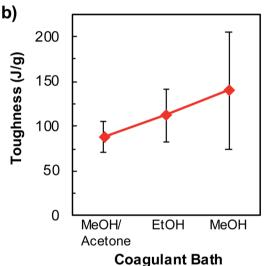
Fig. 5 Mechanical properties including (a) tensile strength, Young's modulus, and (b) toughness of pristine BNNTs/PVA fibers produced from dispersions containing 0.1 mass% BNNTs and 2.5 mass% PVA in different coagulation baths including MeOH, EtOH, and MeOH/ acetone cosolvent of 25 vol% acetone.
