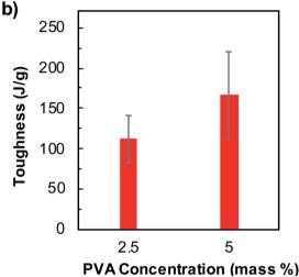
Fig. 4 Mechanical properties including (a) tensile strength, Young's modulus and (b) toughness of pristine BNNTs/PVA fibers produced from dispersions containing 0.1 mass% BNNTs and different PVA concentrations of 2.5 and 5 mass%, respectively, in an EtOH coagulation bath.
