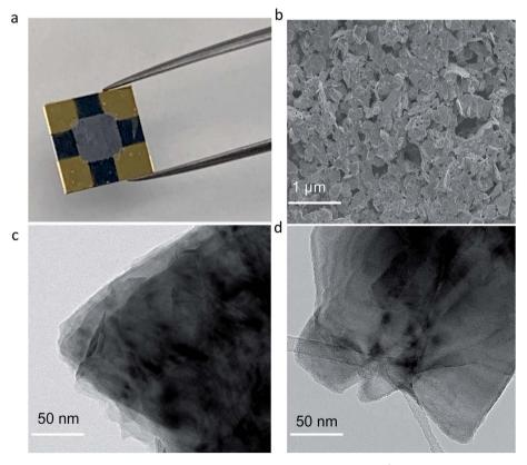
Fig. 2 Surface morphology of MoS<sub>2</sub> samples. (a) Water exfoliated c-MoS<sub>2</sub> (grey area  $\sim$ 7 × 7 mm<sup>2</sup>) on SiO<sub>2</sub> substrate (1 × 1 cm<sup>2</sup>) with Au contacts, and (b) SEM image of water exfoliated c-MoS<sub>2</sub>. The scale bar is 1  $\mu$ m; (c) TEM image of bulk MoS<sub>2</sub>; and (d) TEM image of water exfoliated conductive MoS<sub>2</sub>. Scale bar for both TEM images is 50 nm.
