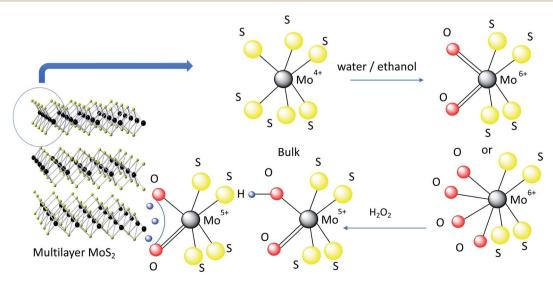
Fig. 5 Schematic representation of the mechanism of formation of conductive MoS<sub>2</sub>.
