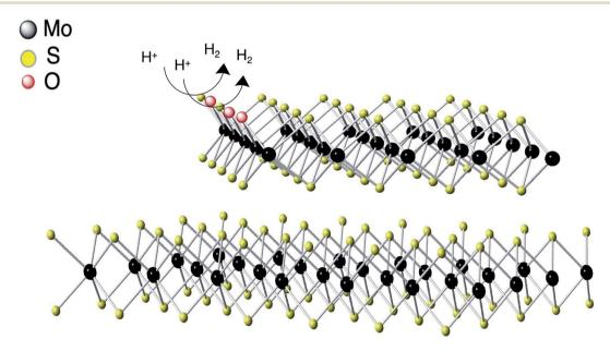
Schematic representation of HER mechanism of conductive MoS<sub>2</sub>. Hydrogen evolution reaction process at the edges of conductive MoS<sub>2</sub>.
