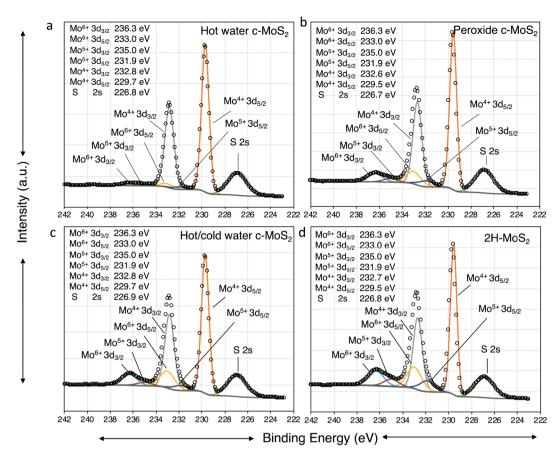
Fig. 4 XPS high resolution spectra of Mo 3d for (a) hot water exfoliated conductive  $MoS_2$ ; (b) peroxide exfoliated conductive  $MoS_2$ ; (c) hot and cold water exfoliated conductive  $MoS_2$ ; and (d) exfoliated semiconducting  $2H-MoS_2$ .
