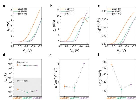
Fig. 2 (a) Transfer, (b) transconductance, and (c)  $I_D^{0.5}$  vs.  $V_G$  curves recorded for p(g2T-TT), p(p2T-TT), and p(b2T-TT). Comparison of the (d) on/off ratios, (e) electronic charge carrier mobilities, and (f) volumetric capacitances measured for the polymers.
