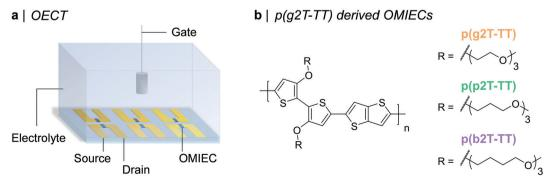
Fig. 1 (a) Schematic representation of an OECT array. (b) Chemical structures of the synthesised OMIECs, namely p(g2T-TT), p(p2T-TT), and p(b2T-TT).
