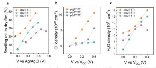
Fig. 3 (a) Polymer swelling relative to the corresponding dry state. Star symbols correspond to the swelling values of the film at  $V_{\rm OC}$  conditions (i.e., passive swelling). The voltage values are plotted vs. Ag/AgCl. (b) Chloride ion and (c) water molecule density in the conjugated polymer film following electrochemical doping at various potentials against VOC. VOC values are 0.14 V for p(g2T-TT), 0.19 V for p(p2T-TT), and 0.35 V for p(b2T-TT).
