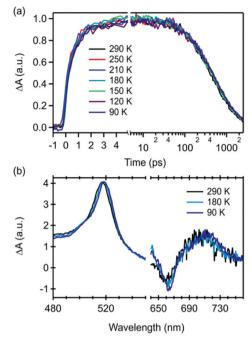
Fig. 4 Transient absorption of 22BP in an inert polystyrene matrix over a range of temperatures 90-290 K. There is no effect of temperature on (a) triplet pair formation and decay and (b) triplet excited state absorption profile
