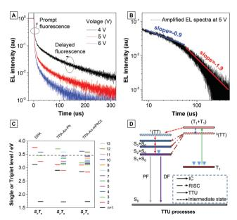
Fig. 5 (A) Transient EL decay of the non-doped device B2 at different voltages. (B) Amplified EL spectra of the non-doped device B2 at 5 V. (C) Energy diagrams. Energy levels and twice the T<sub>1</sub> energies (dashed line) of the anthracene derivatives calculated using B3LYP/6-311G(d,p), where n is the quantum number used to indicate the excited state. (D) Proposed TTU mechanism based on the emitters
