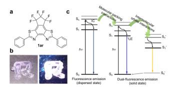
Fig. 1 (a) Molecular structure of 1ar emitting white light in the solid state. (b) Photo-pattern of **1ar** under white light (right) and UV ( $\lambda = 365$  nm, 277 mW cm<sup>-2</sup>) light irradiation (left) at room temperature. The fluorescent molecule 1ar dissolved in chloroform was drawn in an "R" pattern and dried. (c) Jablonski diagram for dual-fluorescence emission of 1ar.
