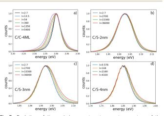
Fig. 3 Evolution of the emission spectra at room temperature of the series of 4 NPLs having different shell thicknesses as a function of excitation intensity at 420 nm. The intensity is expressed in W cm<sup>-2</sup>.
