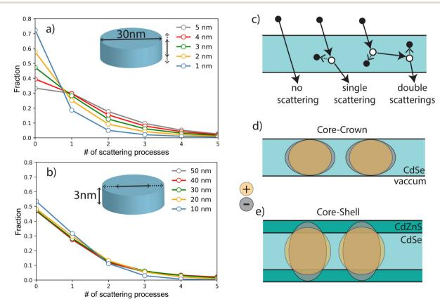
Fig. 8 (a) Distribution of the number of scattering processes in CdSe NPLs when varying the thickness (a), and the lateral size (b). (c) Example of situation with 0, 1 and 2 scattering processes. Schematic charge distribution of holes and electrons in the case of core-crown (d) and core-shell NPLs (e).
