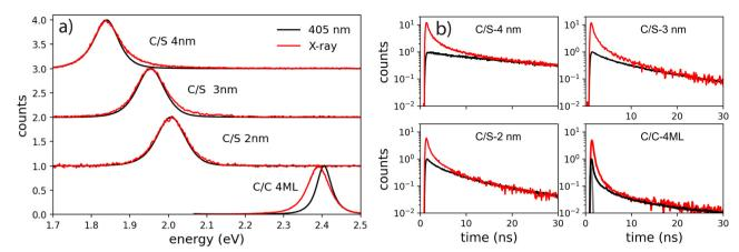
Fig. 6 (a) Emission spectra and (b) fluorescence decay times at room temperature of the series of NPLs having different thicknesses ranging for C/C 4ML (1.2 nm), and C/S 2 nm, 3 nm and 4 nm under low power density of optical excitation (405 nm) and X-ray excitation.
