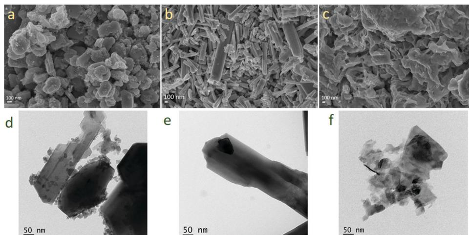
Fig. 7 SEM images of (a) WO<sub>3</sub>, (b) WO<sub>3-x</sub> and (c) WS<sub>2</sub> and TEM images of (d) WO<sub>3</sub>, (e) WO<sub>3-x</sub> and (f) WS<sub>2</sub> after the cycling stability test.
