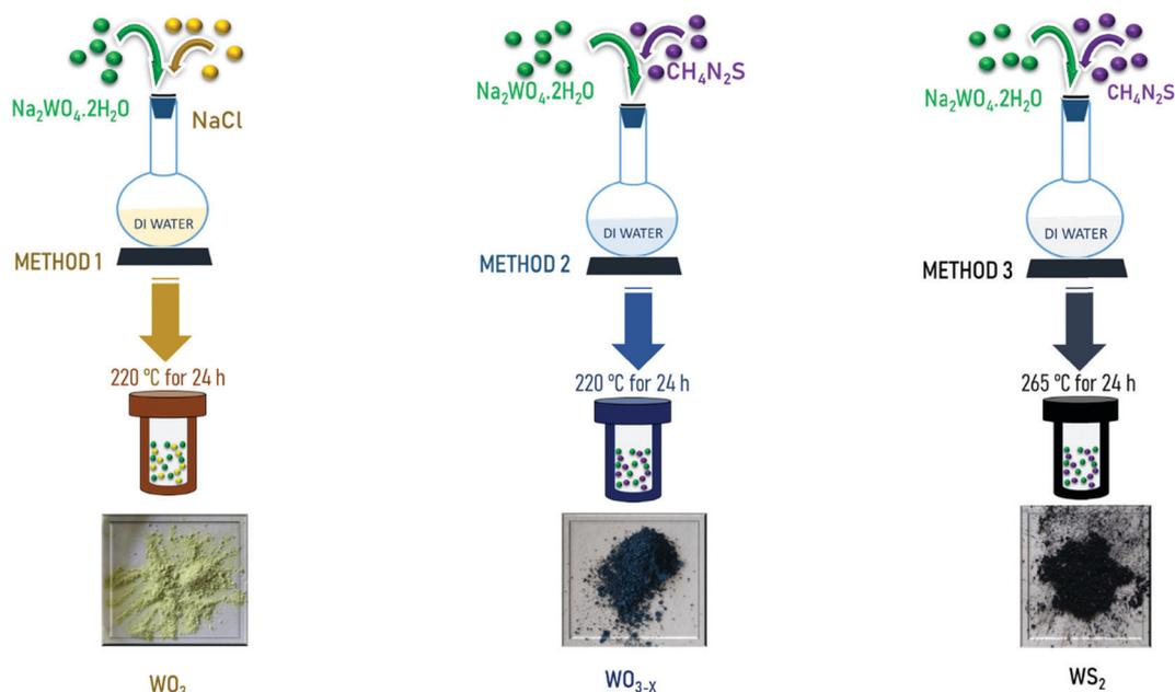
Fig. 1 Schematic of the synthesis of tungsten based nanostructures.
