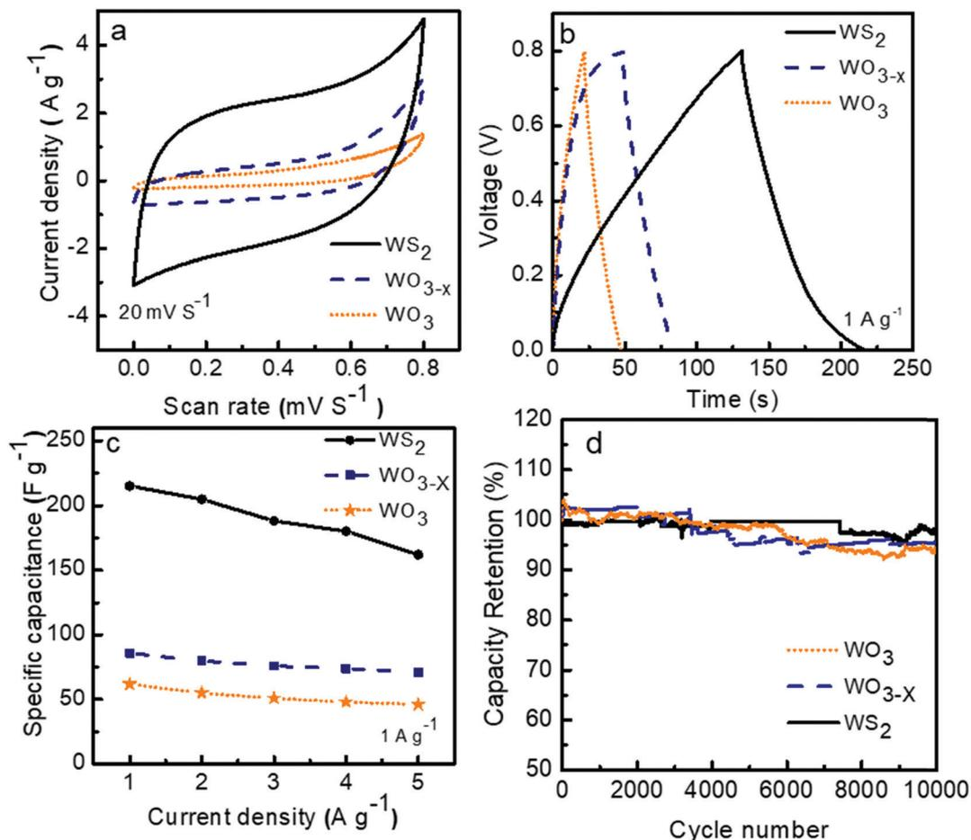
Fig. 6 (a) CV curve of WO<sub>3</sub>, WO<sub>3-x</sub> and WS<sub>2</sub> at 20 mV s<sup>-1</sup>, (b) GCD curve of WO<sub>3</sub>, WO<sub>3-x</sub> and WS<sub>2</sub> at 1 A g<sup>-1</sup>, (c) variation of the specific capacitance with current density, (d) the capacitance retention of the WO<sub>3</sub>, WO<sub>3-x</sub> and WS<sub>2</sub> electrode material over 10 000 cycles.
