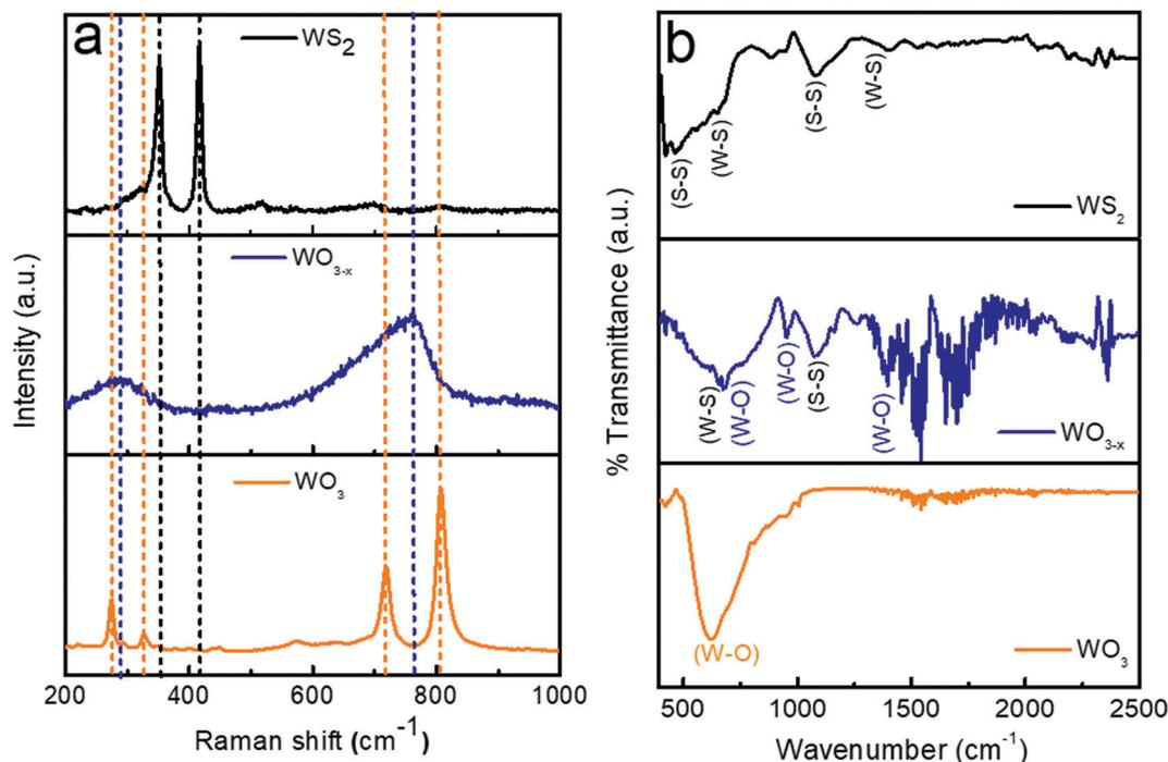
Fig. 3 (a) Raman spectra, and (b) FTIR spectra of the  $\text{WO}_3$ ,  $\text{WO}_{3-x}$  and  $\text{WS}_2$  samples.
