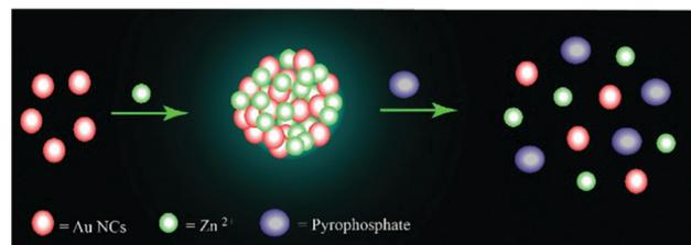
**Scheme 1** Schematic representation of the possible mechanism of quenching of the delayed bright green luminescence of Zn Au NCs upon the addition of sodium pyrophosphate.
