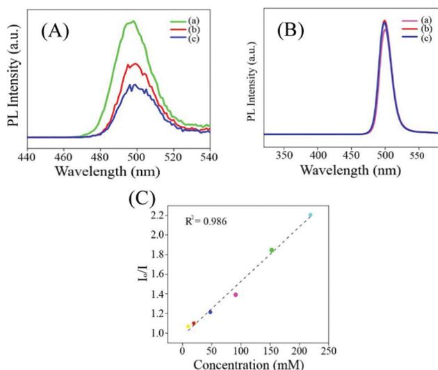
**Fig. 2** (A) Delayed fluorescence emission spectrum of (a) Zn Au NCs and that following the addition of (b) 220  $\mu\text{L}$  and (c) 560  $\mu\text{L}$  addition of 1 M KI solution. (B) Prompt fluorescence emission spectrum of (a) Zn Au NCs and that following the addition of (b) 220  $\mu\text{L}$  and (c) 560  $\mu\text{L}$  addition of 1 M KI solution. (C) Stern Volmer plot calculated based on (A).
