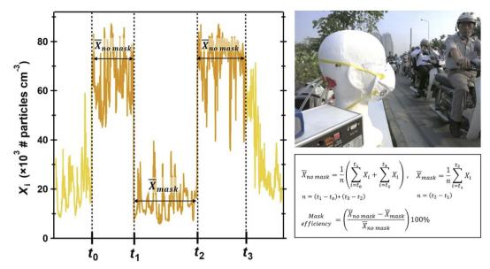
Fig. 3 Mask efficiency tests. The particle instruments were connected by sampling tubes passing from the back to the front (nose area) of the manikin. Each test consisted of three  $\sim$ 10 min sampling periods. The particle concentration without a mask ( $X_{no\ mask}$ ) was obtained in the first and third periods, and the concentration with a mask ( $X_{mask}$ ) during the second period. The total inward leakages of the masks were calculated based on the formulae outlined.
