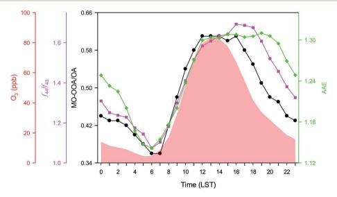
Fig. 6 Diurnal variability of the ambient concentration of O<sub>3</sub> (red shaded area), degree of oxidation obtained as the ratio between ions m/z 44 and 43 ( $f_{44}/f_{43}$ ) measured by ACMS, MO-OOA organic mass fraction (MO-OOA/OA), and absorption Angström exponent (AAE).
