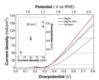
Fig. 6 Linear sweep voltammetry (LSV) recorded at 5 mV s $^{-1}$  in 1 M KOH solution for samples obtained with and without TEA, MgFe-TEA (blue) and MgFe (red), in comparison with an Ni-foam collector (gray). The inset shows the extracted overpotential at 10, 50, and 100 mA cm $^{-2}$  for both samples, MgFe-TEA (blue) and MgFe (red).
