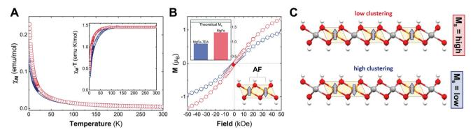
Fig. 4 Magnetic characterization of the MgFe samples with (blue) and without (red) TEA. Magnetic susceptibility as a function of temperature (X<sub>M</sub> vs. T) with an external applied field of 1000 Oe; the inset represents  $(X_M \cdot T \text{ vs. } T)$  (A). Isothermal magnetization recorded at 2 K; the inset depicts the experimental  $M_s$  values in comparison to the theoretical  $M_s$  one (B). Schematic idealized representation of the effect of Fe-clustering over the  $M_s$ values (C).
