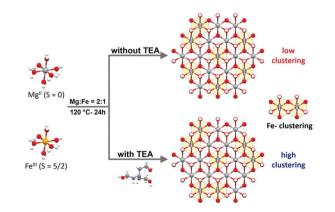
Scheme 1 MgFe-based LDHs (Mg:Fe = 2:1 ratio) are synthesized hydrothermally with ammonia at 120 °C for 24 h. In the case of samples obtained through the TEA approach, a higher Fe-clustering degree is observed which triggers changes in the magnetic behaviour of the final MgFe-based LDHs, even at the same Mg:Fe = 2:1 ratio.
