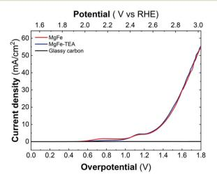
Fig. 5 Linear sweep voltammetry (LSV) recorded at 5 mV s<sup>-1</sup> in 1 M KOH solution by employing glassy carbon collectors for samples obtained with and without TEA, MgFe-TEA (blue) and MgFe (red), in comparison with the bare collector (black).
