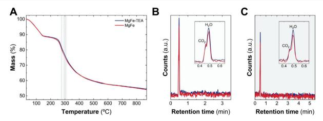
Fig. 2 TG-GC-MS characterization. TG patterns of MgFe-TEA (blue) and MgFe (red) recorded at 10 °C min<sup>-1</sup> under an inert atmosphere of helium (A). During the decomposition process, the evolved gaseous fragments are injected in a preheated GC column at 40 °C. After chromatographic separation, the molecules were identified by MS. Elugrams from the injection at 270 (B) and 300 °C (C) only allow us to identify  $CO_2$  and  $CO_2$  and  $CO_3$  molecules during the decomposition process.
