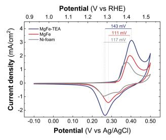
Fig. 7 Cyclic voltammetry recorded at 5 mV s $^{-1}$  between -0.1 V and 0.4 V versus Ag/AgCl for the samples MgFe-TEA (blue) and MgFe (red) and Ni-foam (gray) after 20 cycles of the activation process.
