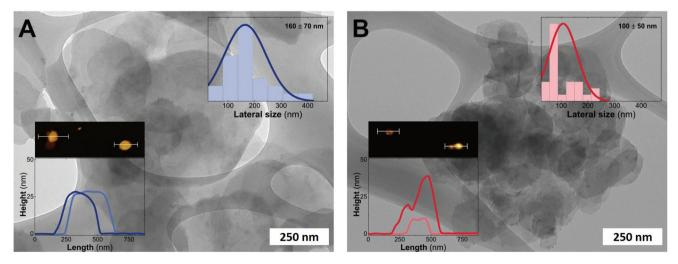
Fig. 3 TEM images of MgFe-based LDHs obtained hydrothermally at 120 °C and a 24 h aging process with and without TEA as the capping agent; MgFe-TEA (A) and MgFe (B), respectively. Insets: Histograms obtained after measuring at least 50 particles. AFM images reveal an estimated thickness lower than 35 nm for both samples.
