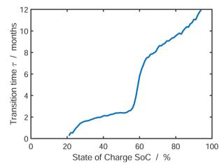
**Fig. 6** Transition time  $\tau$  from dense to porous SEI growth defined as  $L_{\rm in}(\tau) = L_{\rm out}(\tau)$  depending on the state of charge. The results were averaged over 1000 simulations.
