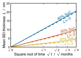
Fig. 2 Growth of the mean SEI thickness  $\bar{L}_{\rm SEI} = 1/A_x \int_0^{A_x} L_{\rm SEI} d\tilde{x}$  over the square root of storage time  $\sqrt{t}$ . Different colors indicate different states of charge. Dashed lines indicate a  $\sqrt{t}$ -growth for comparison.
