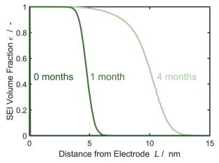
Fig. 4 Evolution of the SEI volume fraction  $\epsilon_{\text{SEI}}$  perpendicular to the electrode over time according to the morphology profiles of Fig. 3, averaged over 1000 simulations. Color gradient indicates increasing storage time from 0 (darkest green) to 4 months (lightest green).
