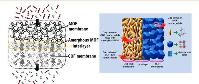
Fig. 3 Schematic representation of MOF/COF composite membrane. The amorphous MOF formed in the interlayer filled the free spaces between COF crystals and the interface between COF and MOF layers. The figure was adapted from the literature with permission from ref. 34. Copyright (2016) American Chemical Society.
