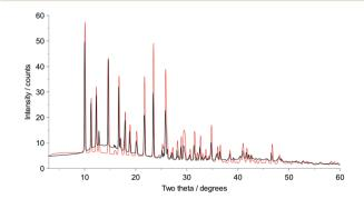
Fig. 2 Capillary PXRD data (black) for cefadroxil monohydrate overlaid upon PXRD data obtained from the equivalent SDPD-SX experiment (red). Note that the y-axis has been arbitrarily scaled to facilitate overlay and does not represent raw counts.
