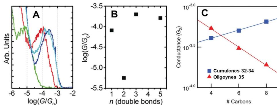
Fig. 14 (A) 1D conductance histograms and (B) conductance values for single-molecule data of cumulenes **30**–**33**. Reproduced with permission from ref. 129 with permission from John Wiley and Sons. (C) Single-molecule conductance values of cumulenes **32**–**34** (blue) and oligoynes **35** (red) as a function of the number of carbons in the chain. Reproduced from ref. 130 with permission from the American Chemical Society.
