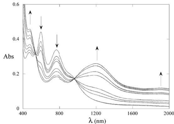
Fig. 18 Spectroelectrochemical reduction (0/–1 states) of complex **51** ( $X = {}^t\text{BuO}$ ) in THF and 0.2 M TBAPF<sub>6</sub>. Reproduced from ref. 150 with permission from the American Chemical Society.
