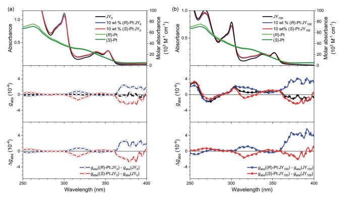
Fig. 4 (a) UV-vis absorption (top),  $g_{abs}$  (middle), and the  $g_{abs}$  difference spectra (bottom;  $\Delta g_{abs}$ ,  $g_{abs}$ (10 wt% Pt:JY<sub>0</sub>) –  $g_{abs}$ (JY<sub>0</sub>)) for the JY<sub>0</sub> films (quartz substrates) in the absence and presence of 10 wt% (R)-Pt or 10 wt% (R)-Pt. (b) UV-vis absorption (top),  $g_{abs}$  (middle), and the  $g_{abs}$  difference spectra (bottom;  $\Delta g_{abs}$ ,  $g_{abs}$ ,  $g_{abs$
