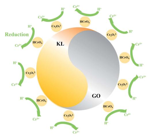
Fig. 6 Schematic diagram of Cr(vi) repair mechanism.
