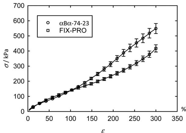
Fig. 4 Average tensile performance for  $\alpha$ B $\alpha$ -74-23 and FIX-PRO® are given as squares and circles respectively, showing similar tensile performance up to 120% strain. Error bars denoting  $\pm$  one standard error at symbols are given for clarity, with lines through data representing the full curve in each case.
