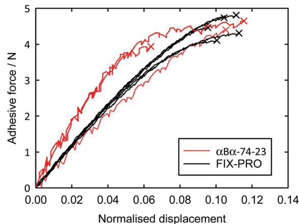
Fig. 5 Adhesive probe tack force as a function of displacement normalised by specimen thickness, for 3 specimens of  $\alpha$ B $\alpha$ -74-23 and for 5 specimens of FIX-PRO®. Crosses indicate failure properties for both materials.
