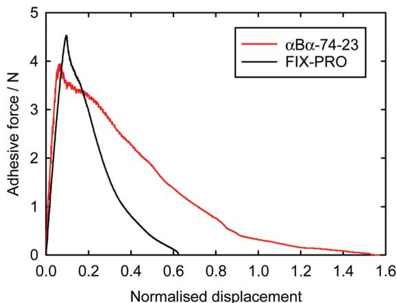
**Fig. 6** Representative probe adhesion results for single specimens of  $\alpha$ B $\alpha$ -74-23 and FIX-PRO<sup>®</sup> to full detachment.  $W = 69.3 \text{ kJ m}^{-3}$  for  $\alpha$ B $\alpha$ -74-23, and  $39.5 \text{ kJ m}^{-3}$  for FIX-PRO<sup>®</sup> were determined from the areas under the curves.
