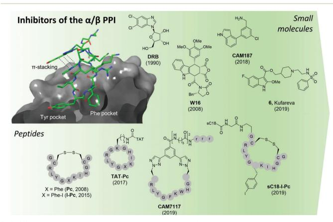
Fig. 9 CK2 inhibitors reported in chronological order and acting at the protein interface between the catalytic and regulatory subunit with the cocrystal structure of CK2 $\alpha$  and CAM7117 shown on the left (PDB: 6Q4Q). The hydrophobic Tyr and Phe pockets key to binding are highlighted, alongside the pi-pi stacking interactions of the ligand.  $sC18 = H_2N-GLRKRLRKFRNKIKEK-NH_2$ ; TAT = GRKKRRQRRRPPQ. Gompounds have been labelled as in the related papers. r = D-Arg.
