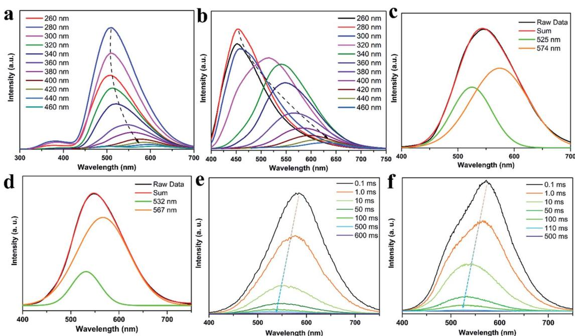
Fig. 6 (a) RTP emission spectra of CDs@IPA and (b) CDs@MA under different excitation wavelengths. (c) The RTP emission spectra of CDs@IPA and (d) CDs@MA at  $\lambda_{\text{ex}} = 360$  nm, and the Gaussian fitted by two emission peaks. (e) Time-resolved emission spectra of CDs@IPA and (f) CDs@MA.
