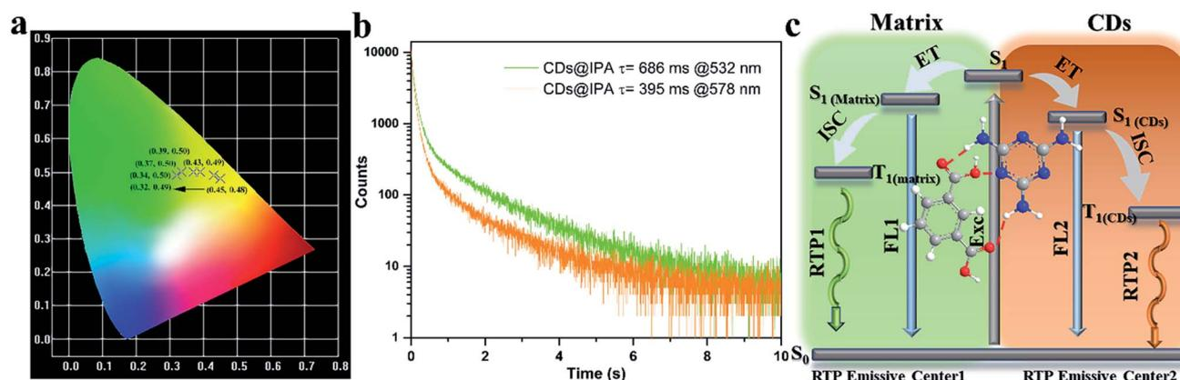
Fig. 7 (a) CIE coordinates of time-dependent colors of CDs@IPA. (b) Corresponding RTP decay profiles of CDs@IPA. (c) The proposed mechanism of time-dependent evolutive RTP colors for the CDs@host matrix.
