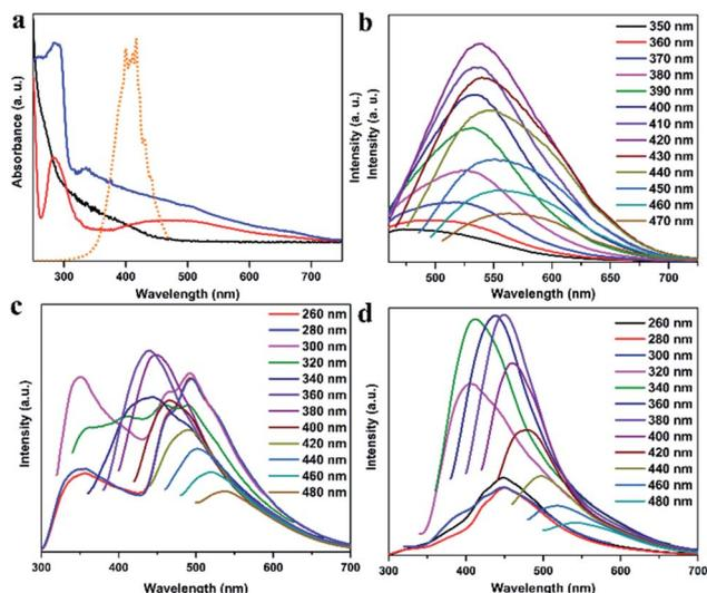
Fig. 3 (a) UV-vis absorbance spectra (black line for CDs, blue line for CDs@IPA and red line for CDs@MA) and FL excitation spectrum of CDs (orange line). FL emission spectra of (b) CDs, (c) CDs@IPA and (d) CDs@MA under different excitation wavelengths.
