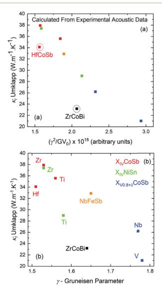
Fig. 3 Plots of calculated lattice thermal conductivity ( $\kappa_{\rm l}$ ) at 300 K (see Section 2.4), assuming the presence of only Umklapp scattering (i.e. for the defect free parent materials), versus (a) the variables determining the magnitude of Umklapp scattering and (b) the acoustic Grüneisen parameter. HfCoSb and ZrCoBi have lower  $\kappa_l$  due to low  $v_s$  (see Table 2).
