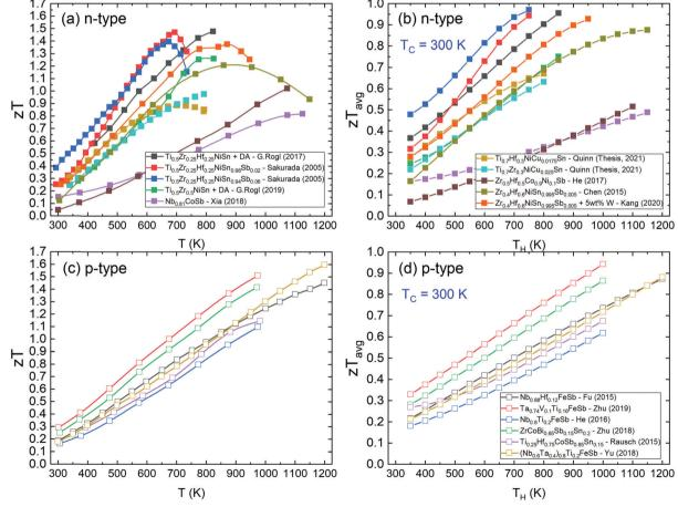
Fig. 4 Literature zT values of the best n-type and p-type half-Heusler thermoelectric materials. Panels (a) and (b) show zT and the average  $zT_{avg}$  of n-type samples as a function of temperature.  $^{142,148,172,174,179,183,191,242}$  Panels (c) and (d) show zT and the average  $zT_{avg}$  of p-type samples.  $^{47,48,75,120,121}$  XNiSn systems have large low temperature zT, but their increase slows above 800 K due to onset of bipolar transport linked to the relatively small band gap.
