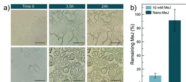
**Fig. 6** (a) Optical micrographs of drops containing MeJ (top) and nano-MeJ (bottom) collected at different time intervals at 50 °C. Scale bar = 100  $\mu\text{m}$ . (b) Percentage of remaining MeJ (quantified by UV-vis spectroscopy) after 24 hours at 50 °C for both treatments.
