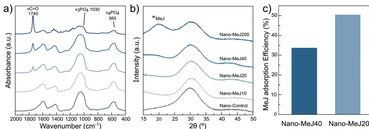
**Fig. 1** (a) FTIR spectra and (b) XRD patterns of ACP nanoparticles (nano-Control) and nano-MeJ synthesized with increasing MeJ concentrations (nano-MeJ10, nano-MeJ20, nano-MeJ40 and nano-MeJ200). (c) MeJ adsorption efficiency for nano-MeJ40 and nano-MeJ20.
