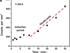
Fig. 3 Two-stage method for measuring nucleation rates in pure FCZ liquid, Form II crystals nucleate at 303 K for 1 and 30 min, followed by 3 min at 373 K (a). Nuclei density as a function of nucleation time at 303 K (b).
