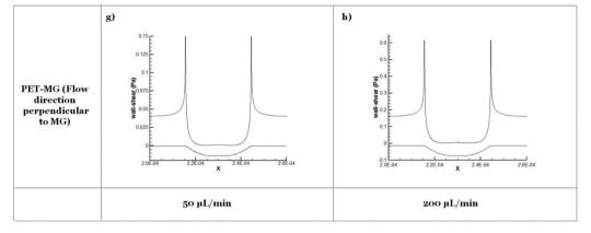
Fig. 6 Contour plots on PET-Flat (a and b) and PET-MG substrates (c and e) and cross-section profiles (dotted line) (d, f, g and h) of computed wall shear stress for 50 (a, c, d and g) and 200  $\mu$ L min<sup>-1</sup> (b, e, f and h) flow rates. Microgrooves are parallel (c-f) or perpendicular (g and h) to the flow direction. Lower curve in d, f, g and h depicts modeled geometry of microgroove cross-section.
