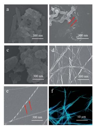
Fig. 3 SEM images of S-TPE-Ph-PEA assemblies in DCM/HEX with different ratios: (a) DCM, (b) 8:2, (c) 3:7, (d) 2:8 and (e) 1:9. (f) Confocal fluorescence microscope image of S-TPE-Ph-PEA assemblies in DCM/HEX with a ratio of 1:9
