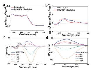
Fig. 2 Absorption spectra (5  $\times$  10<sup>-6</sup> M) (a); CD spectra in solution (b). CD spectra from solid films (c) and circularly polarized luminescence spectra (d) of S-TPE-Ph-PEA assemblies obtained from different solutions: DCM (blue); DCM/HEX 3:7 (cyan); DCM/HEX 2:8 (pink) and DCM/HEX 1:9 (red).
