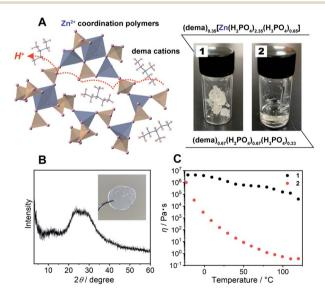
Fig. 1 (A) Schematic structure of 1, the blue and orange polyhedra represent  $\mathrm{Zn^{2+}}$  and  $\mathrm{H_nPO_{4}}$ , the captured organic ions indicate dema cations. The formula and digital photographs of 1 and 2 at 25 °C. (B) The powder X-ray diffraction (PXRD) pattern of 1. The inset shows a digital photograph of a monolith of 1 after annealing at 120 °C. (C) Temperature dependence of the viscosity of 1 (black) and 2 (red).
