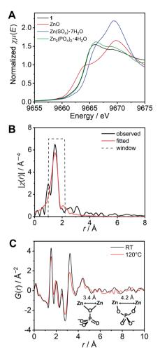
Fig. 2 (A) The XANES region of the XAFS spectra for the  $Zn^{2+}$  K-edge of 1 (black) and references: ZnO (red),  $Zn(SO_4)\cdot 7H_2O$  (blue), and  $Zn_3(PO_4)_2\cdot 4H_2O$  (green). (B) Radial distribution functions (RDF) of 1 (black line) and the fitting curve (red line). (C) The reduced pair distribution function (PDF) profile of 1 and  $Zn^{2+}-Zn^{2+}$  distances.
