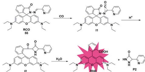
Fig. 8 Sensing mechanism of fluorescent probe 55 .
