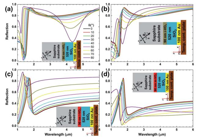
Fig. 5 The angular dependence of infrared reflection when  $VO_2$  is insulator under (a) TE and (b) TM polarized illuminations and when  $VO_2$  is metallic under (c) TE and (d) TM polarized illuminations. The x-z side views of the simulated geometries and illumination conditions are pictured in the insets. The horizontal colored lines in inset (a) stand for incidence angles and apply to all.
