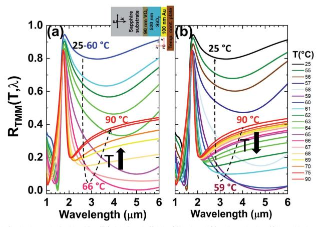
Fig. 6 Simulated spectral reflectivity of  $R_{TMM}(T,\lambda)$  of the "sample C" during (a) heating and (b) cooling cycles. Inset (a) is x-z side view of the simulated "sample C" on the temperature stage and illumination conditions. The dashed black curved lines drawn to guide the eye represent the trajectories of the temperatures during heating and cooling. The colored horizontal lines on the right refer to the temperatures applied during heating and cooling
