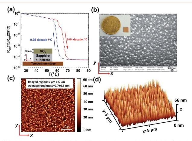
Fig. 1 (a) Electrical characterization of VO<sub>2</sub> ultrathin film ("sample A") as a function of temperature during heating (red colored) and cooling (blue colored). The inset depicts the x-z side view of the "sample A" on a temperature stage. (b) Scanning electron microscope image of the "sample A". Inset: Optical image of the "sample A" and size comparison with a coin of 10 eurocents. (c) 2D and (d) 3D atomic force microscopy images of the "sample A".
