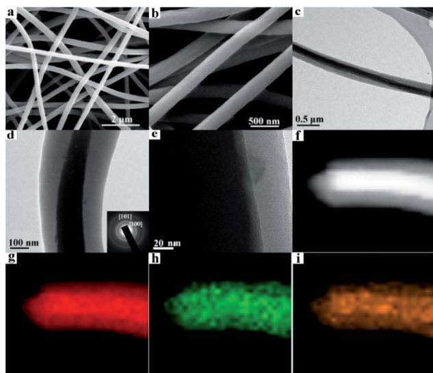
Fig. 1 (a and b) SEM images of GeO<sub>2</sub>/nanocable at low and high magnifications. (c and d) TEM and (e) HRTEM images of GeO<sub>2</sub>/nanocable, inset of (d) is the corresponding SAED patterns; (f) dark field STEM image and (g–i) EDS-elemental mapping images of a single GeO<sub>2</sub>/nanocable (images g, h and i represent C, O and Ge elements, respectively).
