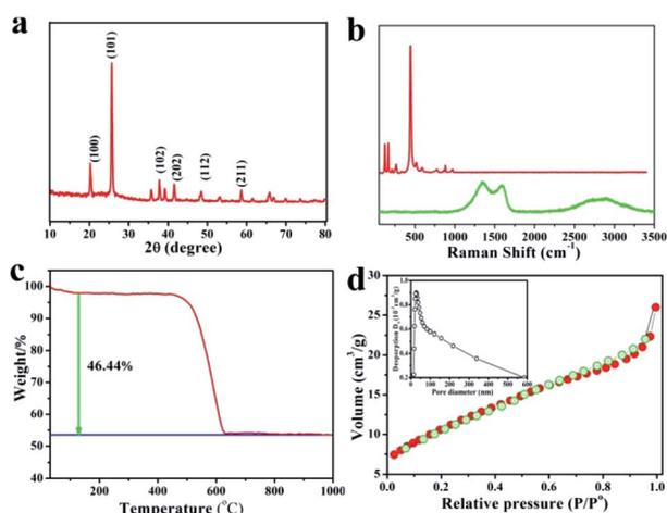
Fig. 3 (a) XRD pattern of GeO<sub>2</sub>/nanocable, (b) Raman spectra of GeO<sub>2</sub>/nanocable (green line) and commercial GeO<sub>2</sub> powder (red line), (c) TG curve of GeO<sub>2</sub>/nanocable in oxygen atmosphere, (d) nitrogen adsorption and desorption isotherms of GeO<sub>2</sub>/nanocable, inset image is the corresponding pore size distribution plots.
