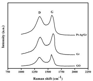
Fig. 3 Raman spectra of GO, Gr and Pt-Ag/Gr.
