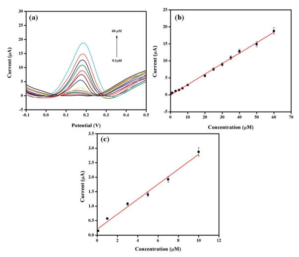
Fig. 6 (a) Differential pulse voltammograms with various DA concentrations (0.1, 1, 3, 5, 7 10, 20, 25, 30, 35, 40, 50, 60 μΜ) at Pt-Ag/Gr/GCE in 0.1 mol L<sup>-1</sup> PBS at pH 6.5. (b) Relationship between peak current and DA concentration. (c) The calibration curve in low concentration range.
