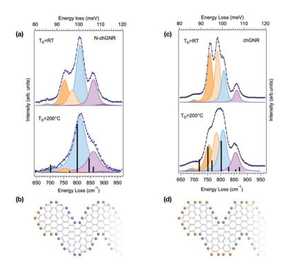
Fig. 3 Comparison between the HREEL spectra of N-doped (a) and pristine (c) chevron-type GNRs, obtained by deposition at T<sub>D</sub> = 200 °C and at RT. The corresponding fitting components are shown as shaded curves, while calculated modes are displayed as black bars. The corresponding molecular schemes, showing the structure of the termini, are reported in (b) and (d), respectively. The top spectrum in (a) is also reported in the right panel of Fig. 1.
