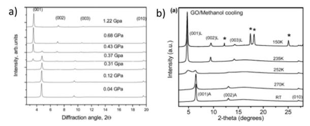
Fig. 10 Pressure (a) and temperature (b) induced phase transition from the ambient 1-layer Brodie GO-methanol structure to a 2-layer structure. (a) XRD patterns ( $\lambda = 0.7092$  Å) recorded from Brodie GO immersed in excess of liquid methanol upon pressure increase. 112 (b) XRD patterns recorded in the process of cooling ( $\lambda = 0.99874 \text{ Å}$ ).<sup>209</sup>
