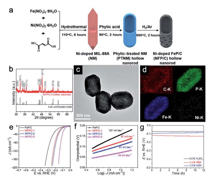
Fig. 7 (a) Schematic illustration of the formation of NFP/C hollow nanorods. (b) XRD pattern, (c) TEM image and (d) EDX mapping images of NFP/C hollow nanorods. (e) LSV plots and (f) Tafel plots of NFP/C hollow nanorods with different Ni/Fe ratios in acid. (g) Durability test of NFP/C in acidic, neutral, and alkaline solutions. Reproduced with permission. 61 Copyright 2019, The American Association for the Advancement of Science.
