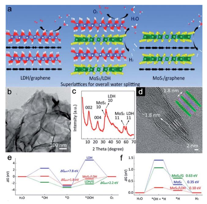
Fig. 4 (a) Schematic diagram of  $MoS_2/LDH$  and control samples for different processes in water splitting. (b) TEM image, (c) XRD pattern, and (d) HRTEM image of the  $MoS_2/LDH$  sample. Free energy illustrations of (e) the OER and (f) HER on  $MoS_2/LDH$  and control samples. Reproduced with permission. <sup>54</sup> Copyright 2019, American Chemical Society.
