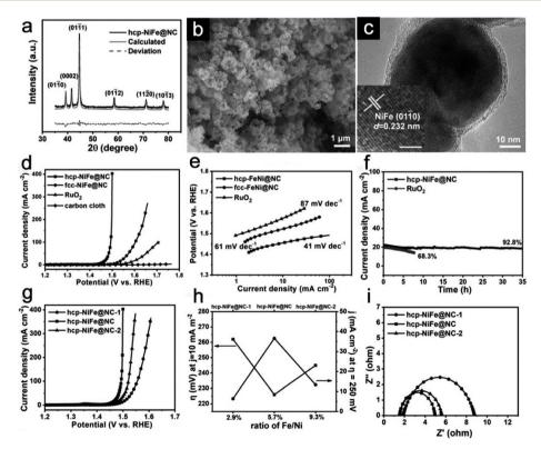
Fig. 5 (a) XRD patterns, (b) SEM image, and (c) TEM image of hcp-NiFe@NC, (d) LSV curves and (e) Tafel plots of catalysts with different phases. (f) I-t curves of the hcp-Ni-Fe@NC and RuO<sub>2</sub>. (g) LSV curves of NiFe alloys with different Fe/Ni ratios. (h) OER performances of NiFe alloy samples at the current density of 10 mA cm<sup>-2</sup> and the  $\eta$  of 250 mV. (i) Nyquist plots of NiFe alloy samples. Reproduced with permission.<sup>55</sup> Copyright 2019, John Wiley & Sons, Inc.
