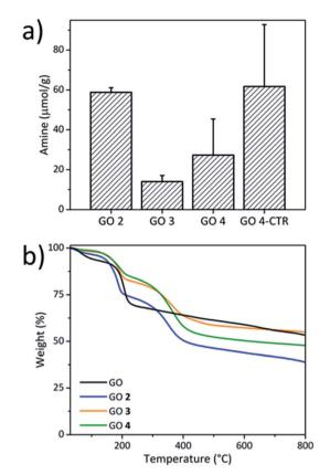
Fig. 3 (a) Kaiser test of GO 2, GO 3, GO 4 and GO 4-CTR, and (b) TGA of the pristine GO, GO 2, GO 3 and GO 4 performed in an inert atmosphere.
