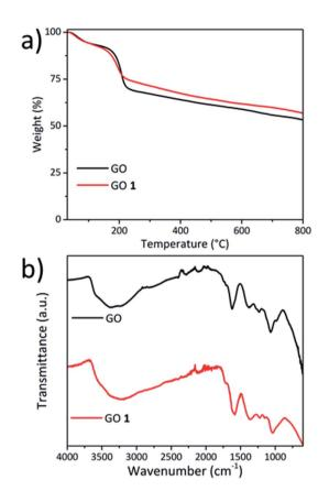
Fig. 2 (a) TGA of the pristine GO and GO 1 performed in an inert atmosphere. (b) FT-IR spectra of the pristine GO and GO 1.
