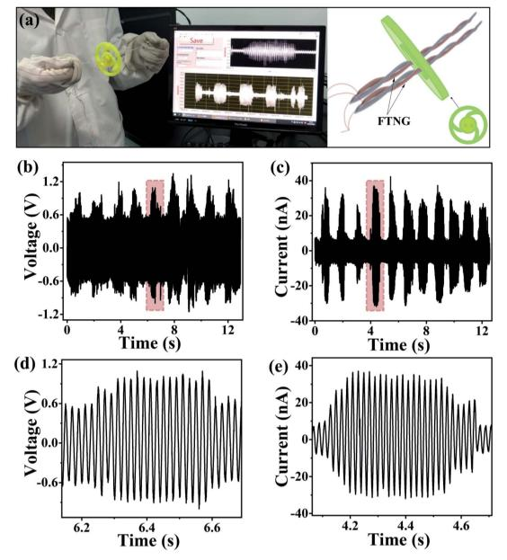
(a) Schematic of the application of FTNG on harvesting the spinning energy. (b) Output voltage and (c) output current of FTNG driven by the spinning movement. The corresponding enlarged view for one wave packet of the output voltage (d) and output current (e).
