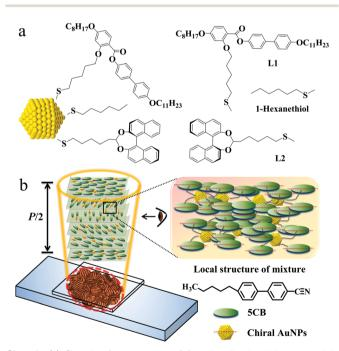
Chart 1 (a) Sketch of a segment of functionalized gold nanoparticle ChirAuLC, (b) cartoon introducing the concept of induced chiral structure in host 5CB by the macro-chiral liquid crystal nanoparticles (ChirAuLC).
