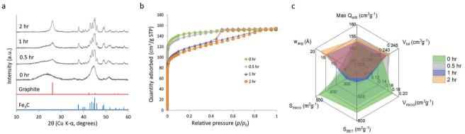
Fig. 7 (a) XRD diffraction patterns for carbons synthesized from starch (5 g) and iron nitrate (3.4 mmol) and held at 800 °C for different times. (b) N<sub>2</sub> adsorption isotherms and (c) adsorptive characteristics of these starch-derived carbons.
