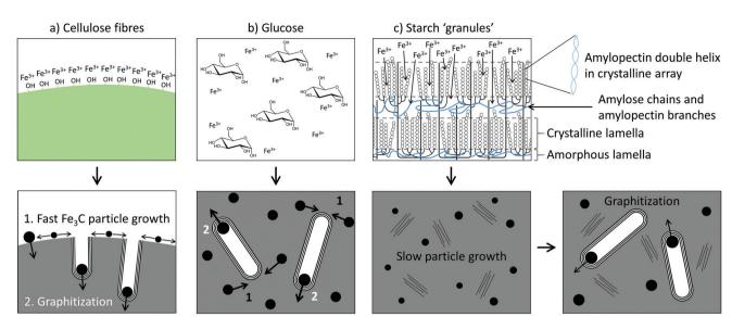
Fig. 8 Schematics of the mechanism of graphitization for (a) cellulose fibres, (b) glucose and (c) starch.
