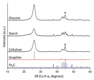
Fig. 2 PXRD patterns for carbon/Fe $_3$ C samples produced from glucose, starch and cellulose (5 g) and iron nitrate (0.68 mmol), held at 800  $^{\circ}$ C for 1 h. (\*) indicates presence of minor  $\alpha$ -Fe phase.
