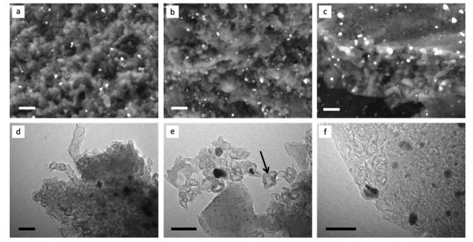
Fig. 3 SEM images (backscattered electron detector) of porous carbons derived from (a) glucose, (b) starch and (c) cellulose (5 g) and iron nitrate (0.68 mmol), held at 800 °C for 1 h (scale bar = 200 nm) and TEM images of the carbons derived from (d) glucose, (e) starch and (f) cellulose (scale bar = 100 nm)
