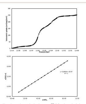
Fig. 12 N<sub>2</sub> volumetric uptake isotherm at 77 K for the calculation of the BET surface area of NUIG1 (top), and plot of the selected linear region that that satisfies the consistency criterion (bottom). 48
