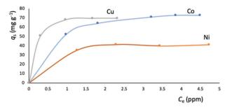
Fig. 8 Equilibrium data for the metal adsorption by **NUIG1** (contact time: 30 min). The solid lines are a quide to the eye.
