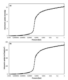
Fig. 13 Gravimetric (top) and volumetric (bottom) uptake isotherms for NO at 121 K.
