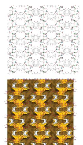
Fig. 2 Representation of the 3d structure of **NUIG1** along the a axis (top) and its pore network shown in yellow (bottom). Color code: N (dark blue), Zn (light blue), Na (green), O (red), C (grey).
