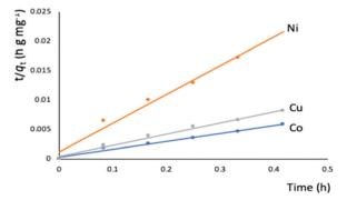
Fig. 7 Top: Metal adsorption capacity (mg  $g^{-1}$ ) versus time (h) plot. The solid lines is a guide to the eye; bottom: simulation of the experimental data to the pseudo-second order kinetic model. The solid lines represent the fitting of the data.
